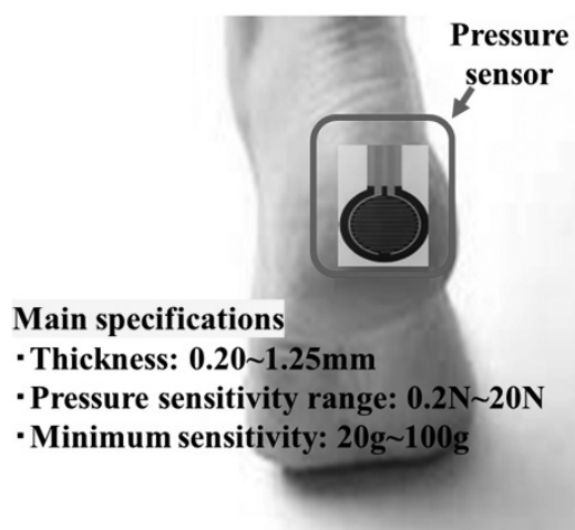
Figure 7 : Pressure sensor installation site.
